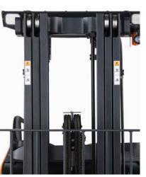
**High Visibility Mast** Neatly arranged hydraulic hosing and strategic placement of chains provide excellent visibility.
