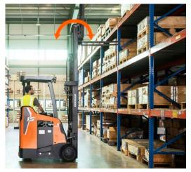
**Auto Tilt Leveling** Returns the mast back to vertical position via tilt angle sensor.
