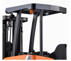
**3-Post Overhead Guard** Outer mast aligned with front legs improve operator safety.
